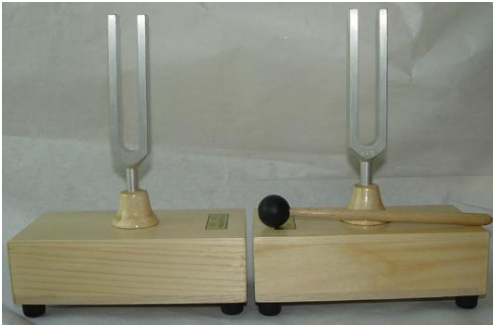
Beat frequency experiment on tuning fork
